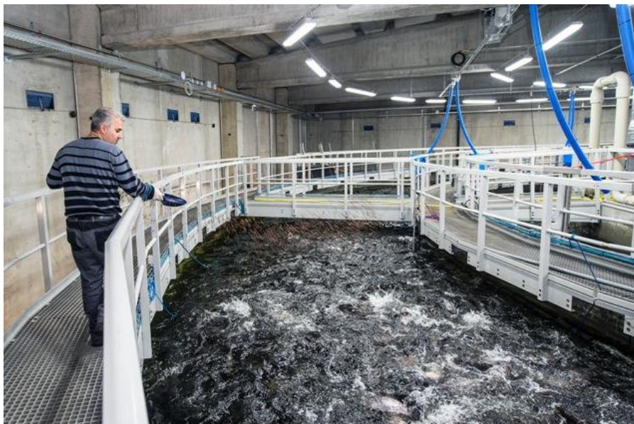
Figure 6: A large round tank (6 m deep, 32.5 m in diameter) as part of a salmon RAS ( Swiss Alpine Fish )
